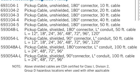
CSA-certified Altronic components. The standard cables have 50' of PU cable, and the "A" suffix variation has 100' of PU cable.
