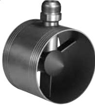
low restriction air-gas mixer ensures that adequate air-flow is maintained to the engine and that operating efficiencies are not compromised by installation of the device. The computer-aided-design mixer is built to aerospace tolerances using CNC machining processes and is assembled using state-of-the-art welding techniques. The finished mixer has no moving parts and once installed in the engine air-intake system requires no routine maintenance.
